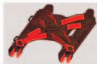
Reinforced track frame sections (shown in red)
