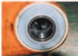
WC Thermal Spraying (Tungsten Carbide)
