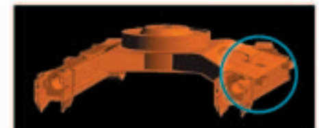
Undercarriage Designed for Easy Mud Removal
