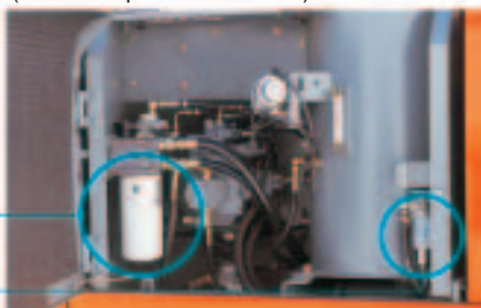
Engine Oil Filter and Water Separator Positioned for Easy Checking from Ground
